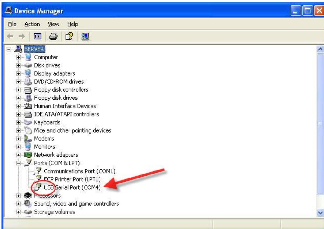
It is most likely your newer PC's today do not have enough COM ports so Steltronic has included with your PC some Com Port conversion devices. These devices plug into the USB port of your computer and they create a COM port inside of Windows.
