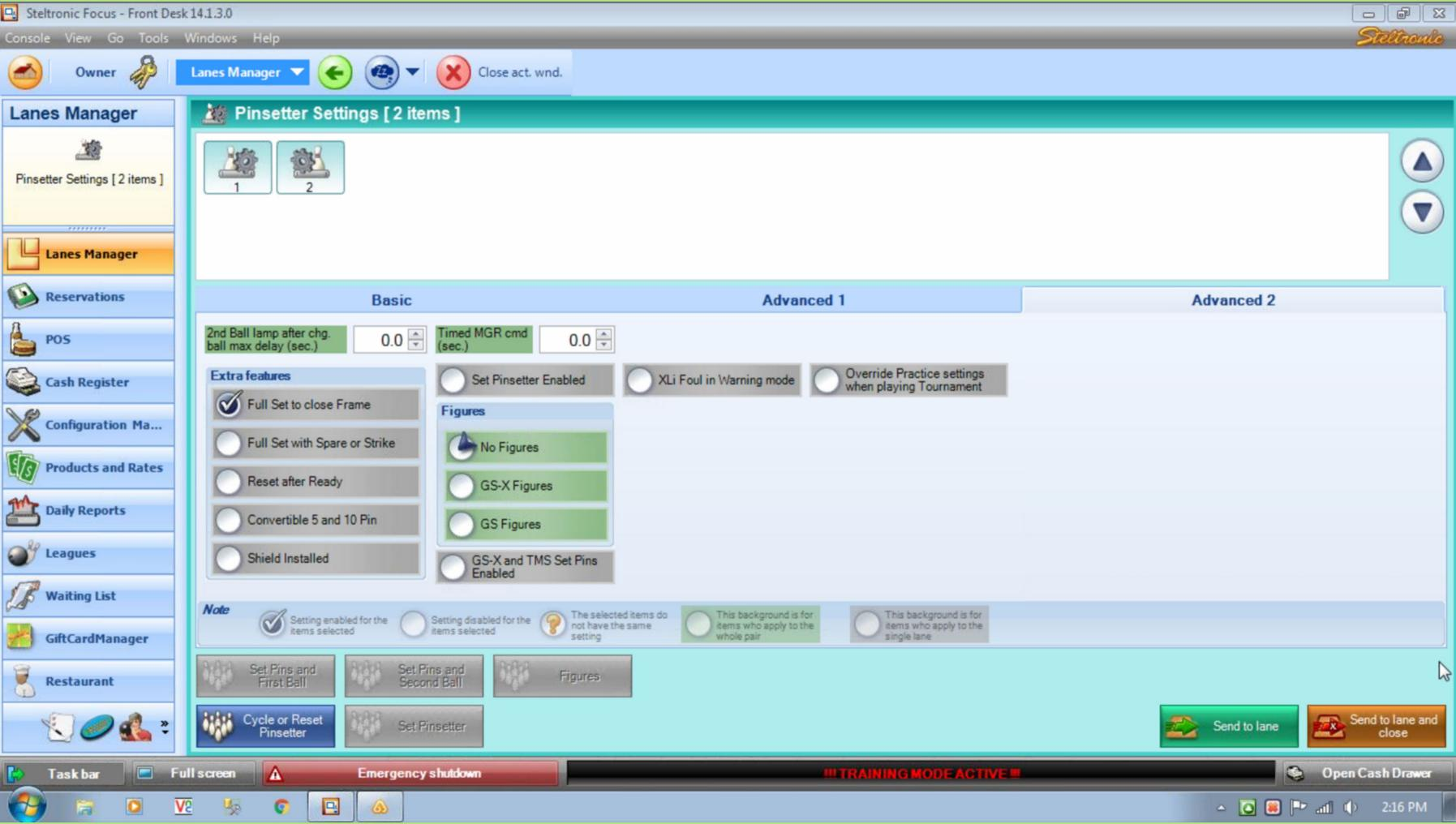
Using Focus, click the configuration manager, then scroll to the pinsetters tab, then find your exact pinsetter in the list of pinsetters.
