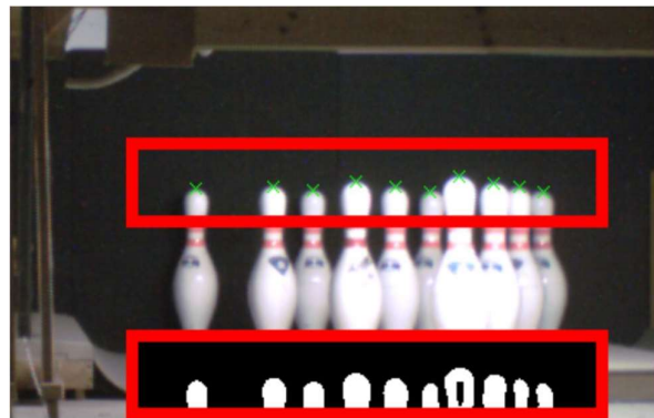
Calibration is succesful but the light is too much; the camera could see pins even when knocked down. Lower the exposure level
