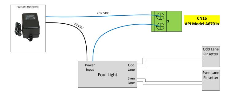
If you cut the 12 volt line (low voltage) output of the transformer, you are essentially going to control the power being supplied to the foul light.
