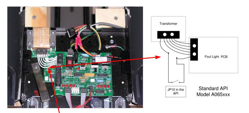
If you cut this white wire on the transformer, you are essentially cutting off the low voltage to the foul light.
