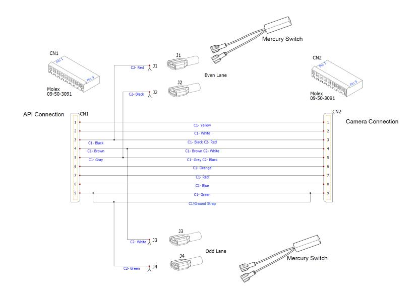
Odd Lane Mercury Switch: When connecting the mercury switch to the camera cable, the ODD lane mercury switch should be connected to the white and green wires on the camera cable with quick disconnects.
