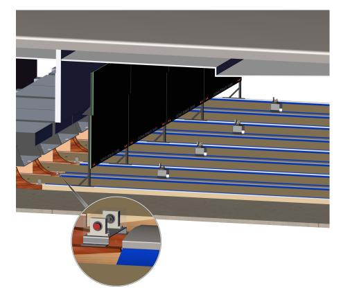
The PinCam also has infrared sensors that detect a bowling ball. When the bowling ball breaks the "infrared beam", this informs the scoring system that a ball was rolled, and then to detect the standing pins for a score.
