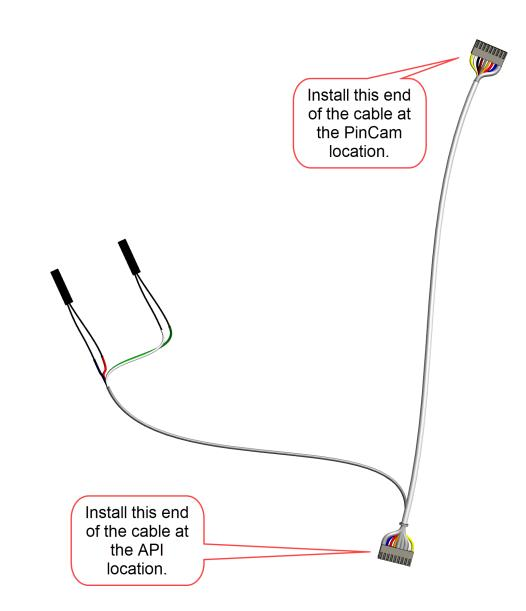
Steltronic has also supplied a special camera cable that has extra connections for the mercury switches. When you install the camera cable (PN - 716005-SPECIAL), please make sure you have installed the cable that has the quick disconnects closest to the API on the curtain wall.
