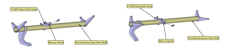
Mercury switch installed with rake UP and pinsetter at zero degrees.
