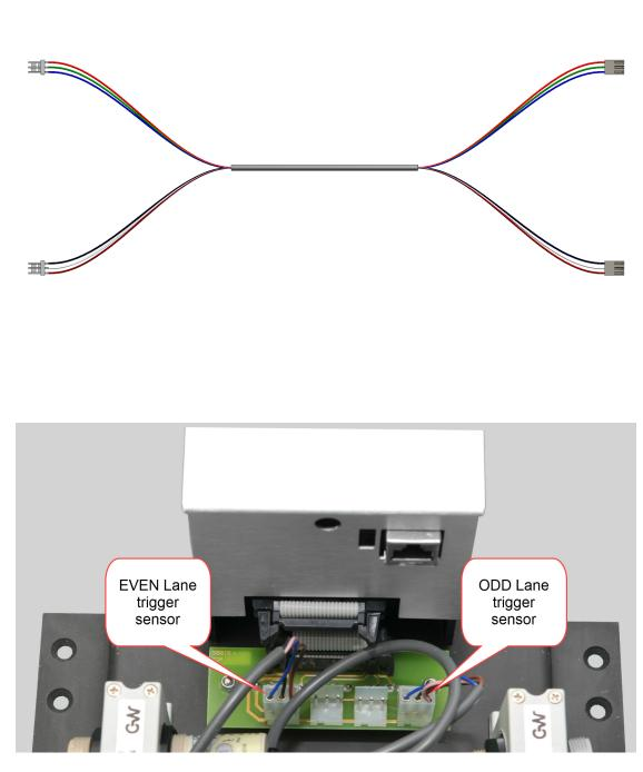
When you have installed the sensors onto the new bracket and mounted them under the ball return tracks, you need to connect these sensors back onto the PinCam.
