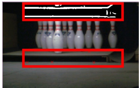
Calibration failed because the Camera is looking too low.
